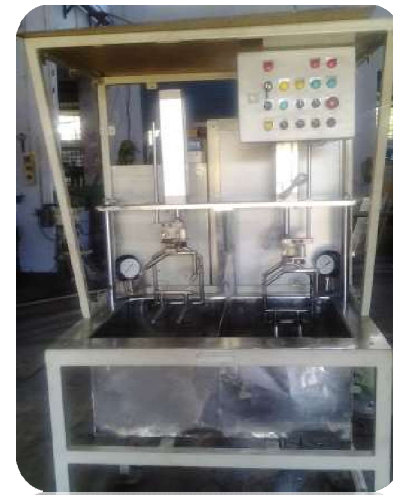
Machine Name – Fuel Tank Leakage Testing Machine Type – Testing Machine Customer – Suzuki Two Wheeler
